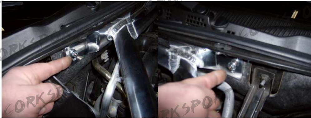
Step 9: Tighten nuts on fire wall to 16-22ft/lbs.
