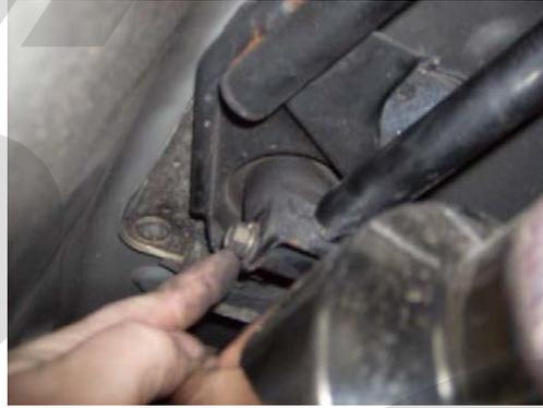
**Step 18:** If your vehicle was equipped with a heat shield reinstall the four 10mm headed bolts to secure the heat shield to your vehicle.
