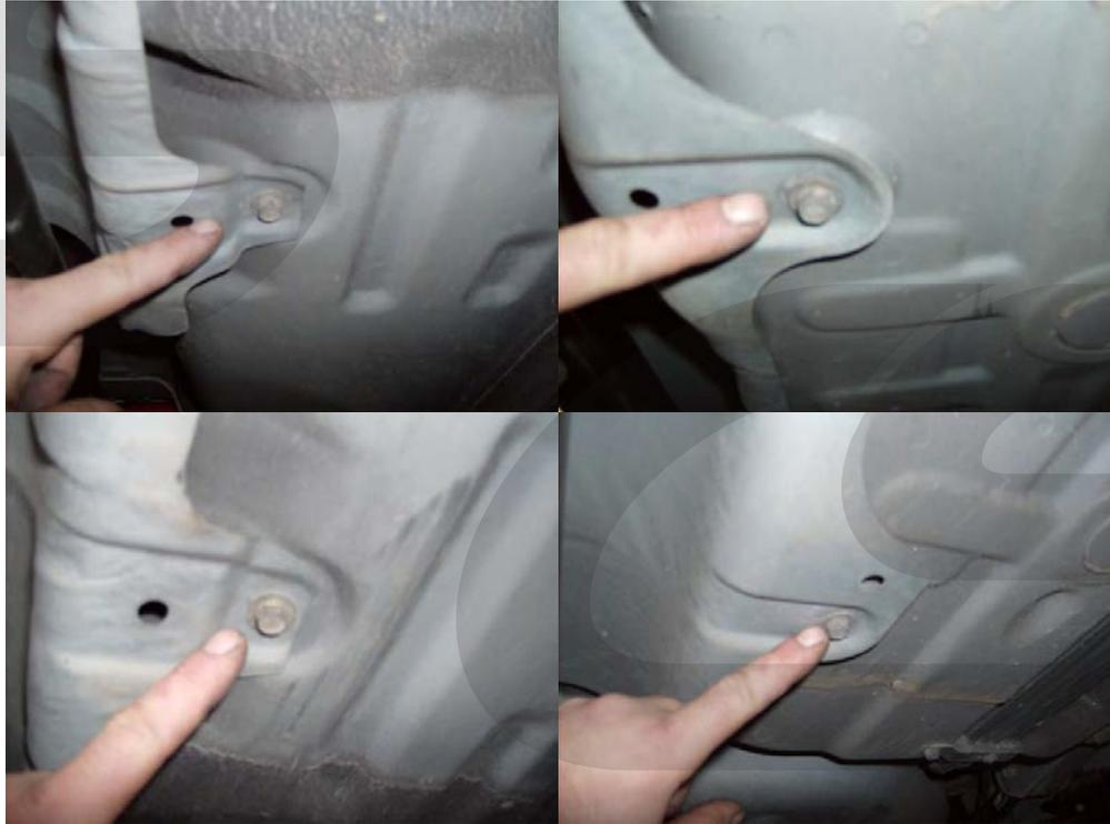
**Step 6:** Slide the heat shield toward the rear of the car several inches to gain access to the shifter.
