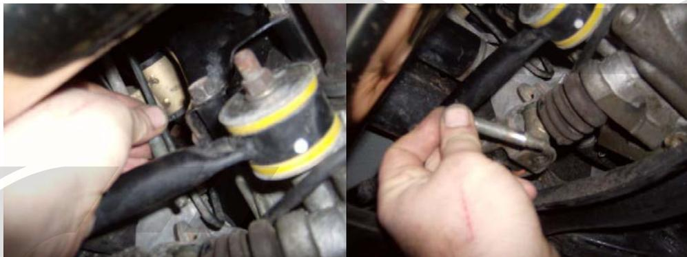
**Step 4:** Slide the shift linkage back from the transmission.
