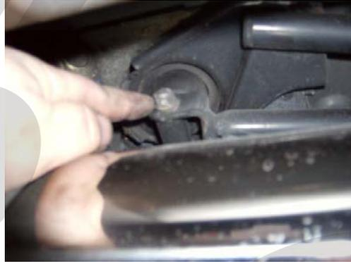
**Step 8:** Remove the 12mm headed bolt from the shifter and the linkage and slide the linkage from the shifter. This will free up the entire shift rod to be removed from the car. Slide it backward and out of the car (once it clears the front subframe, it will be free to come out around the side of the exhaust piping.)
