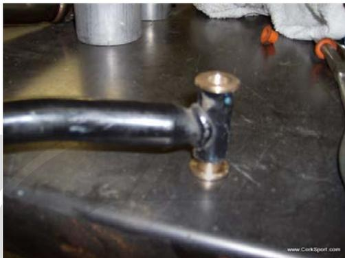
**Step 12:** Install the shift rod into the bracket and install the supplied bolt and nut. Add a small amount of grease between the surface of the bushings and the surface of the bracket. Torque the bolt to 12 ft lbs. Test fit by pivoting the bracket with the drift used to remove the rivet. If the assembly is extremely tight, back the torque off a bit.
