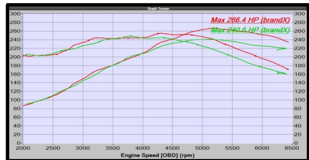
Power/Torque Factory Camshaft vs CorkSport Camshaft
