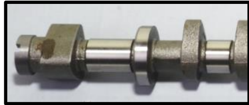
Blank Camshaft with Bearing Surfaces Ground
