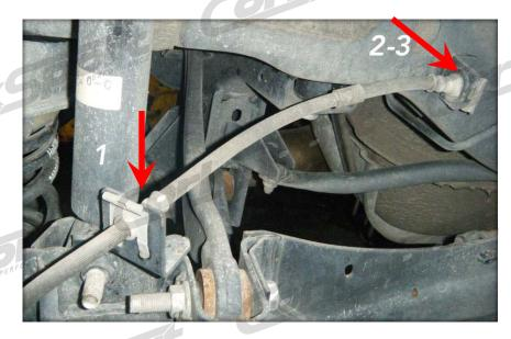
Step 4: Locate the junction for the brake line to the car body. It will take a 10mm wrench to loosen the fitting. (#2 in the picture above) Once the fitting it loose remove the line holder clip (#3 in the picture above).
