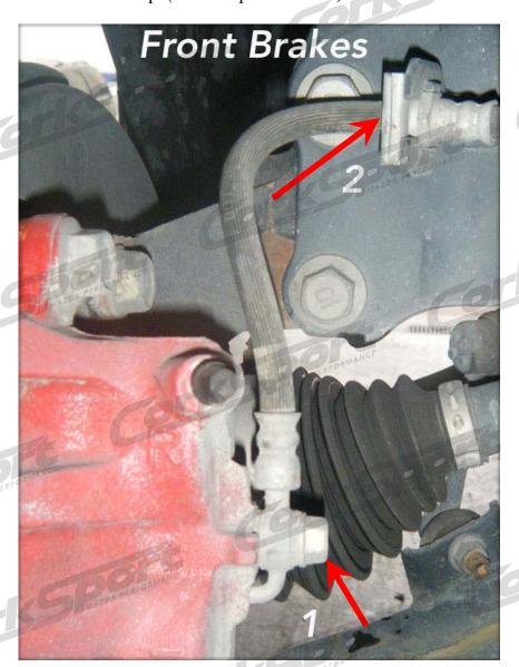
Step 5: Locate the junction for the brake line to the car body. It will take a 10mm wrench to loosen the fitting. (#1 in the picture below) Once the fitting it loose remove the line holder clip. (#2 in the picture below).
