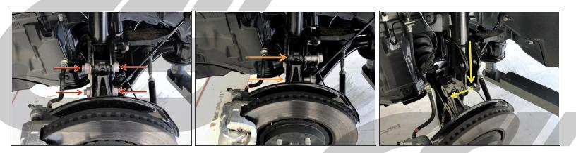
Using a 21mm wrench and 23mm socket with a breaker bar or impact, loosen the lower strut mounting bolts.
