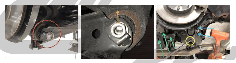
A Do not perform the next step until you are confident the lower control arm bolt is secure.
