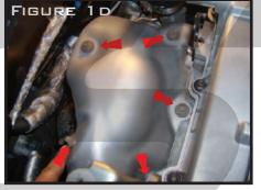
WHEN REMOVING THE SENSOR. YOU CAN DISCONNECT IT AT THE PLUG IF NECESSARY, BUT THERE IS PLENTY OF SLACK TO REMOVE THE SENSOR AND AVOID TWISTING THE CABLE.
