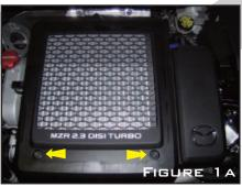
A. REMOVE THE TWO 10MM HEX BOLTS HOLDING THE INTERCOOLER COVER TO THE INTAKE MANIFOLD AS SHOWN IN FIGURE 1A. SLIDE THE INTERCOOLER COVER OFF THE BACK OF THE INTERCOOLER AND OUT OF THE ENGINE COMPARTMENT.
