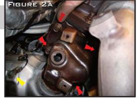
B. Remove 10mm hex head bolt and 02 sensor wiring harness loom from downpipe shown with yellow arrow in Figure 2a. It will be reused to secure the Factory 02 sensor wiring harness.
