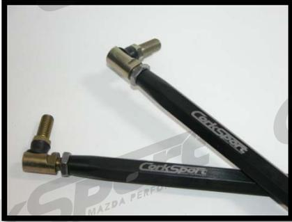
**Thank you for purchasing the CorkSport Mazdaspeed Front Adjustable End Links.** Made to fit OEM and aftermarket front sway bars, the CorkSport Mazdaspeed 3 Front Adjustable End Links allows customers to tune any sway bar and remove the preload commonly associated with the suspension. We hope you enjoy your purchase. Please let us know your feedback by submitting a review at <http://www.corksport.com/corksport-mazdaspeed-3-front-adjustable-swaybar-end-links.html>
