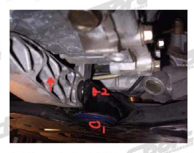
Step 2: Install the inserts in the mount and re install the mount. Tighten the bolts to 70 lb/ft.
