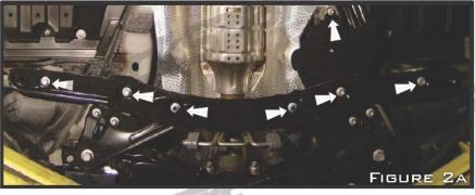
A) REMOVE THE FRONT CHASSIS CROSSMEMBER BY REMOVING THE FASTENERS SHOWN IN FIGURE 2A: 4x 14mm Bolts, 2x 14mm Nuts and 1x 10mm Bolt Holding Brake Line Sheild to the Chassis.
