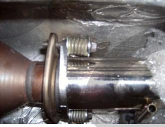
Once the spring is snug with a small amount of gap between the coils use the supplied M10 nut to tighten against the factory catalyst nut to keep the bolt from coming loose.
