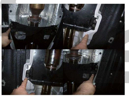
Step 3: Remove the two 14mm headed nuts and two springs from the front of the exhaust system to the mid pipe.
