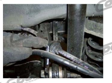
Step 4: Once the line is free from the body and holder loosen the brake line from the caliper. This will take the 14mm wrench. This will allow you to remove the stock brake line.
