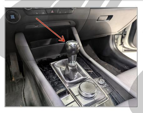
Start by removing the stock shift knob by unscrewing it counterclockwise from the shifter
