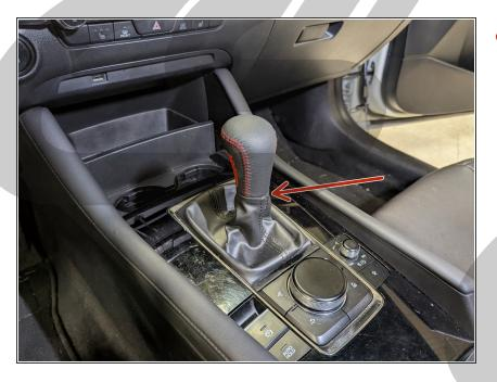
Install the CorkSport Leather Shift Knob onto the shifter and tighten until it meets up with the shift boot
