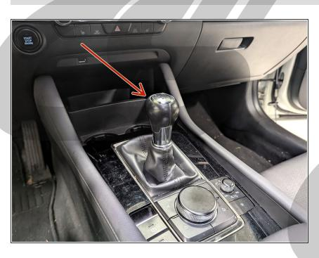
Install the shift knob onto the shifter and tighten until it meets up with the shift boot and is snug
