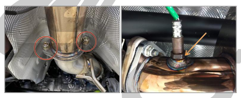
• Line up the downpipe flange, midpipe flange, and crush gasket so they are all centered with each other
