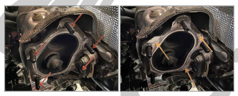
Install the supplied CorkSport studs with the shorter end threaded into the turbocharger. Hand tight
