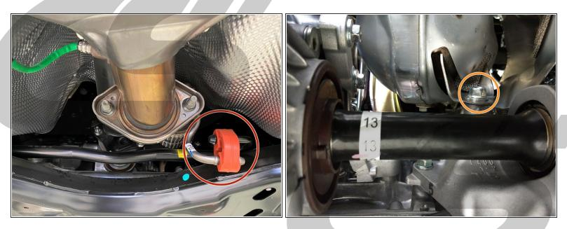
Remove the downpipe exhaust hanger from the rubber hanger on the chassis using exhaust hanger pliers or channel lock pliers
