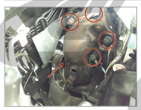
▲ The OEM nuts that secure the downpipe to the turbocharger are "crimp" nuts. They will be difficult to remove and may pull the studs out with the nuts. We recommend spraying some penetrating fluid on the nuts and letting it sit for 30+ minutes to help with loosening
