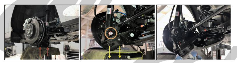
Place the hydraulic jack directly below the driver's side end of the torsion beam and apply a small amount of upward pressure.
