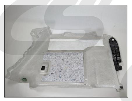
This step is included to give you a reference for tab and clip locations for the trim piece that is removed in the next step
