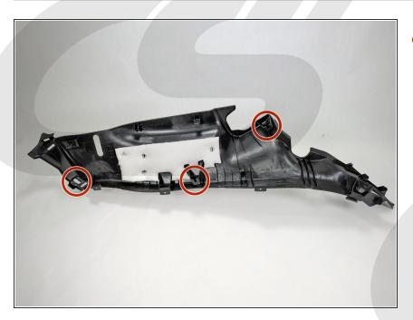
This step is included to give you a reference for clip locations for the trim piece that is removed in the next step
