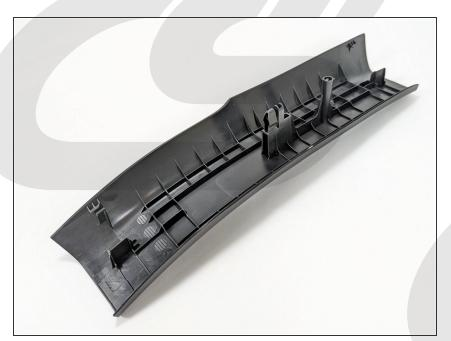
This step is included to give you a reference for tab and clip locations for the trim piece that is removed in the next step
