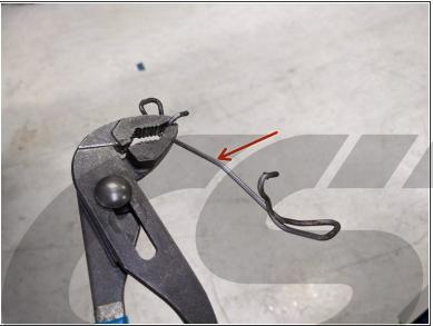
Remove the Spring Clip from the Brake Caliper with a pair of pliers. Pull outward, away from the vehicle
