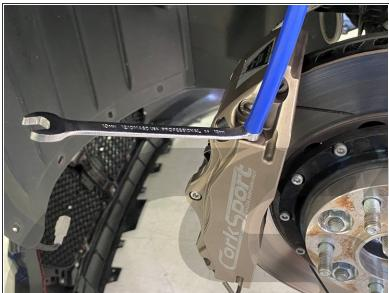
For proper brake bleeding, always start with the bleed screw **furthest** from the master cylinder. In this case we start with the **outer** bleed screw on the **passenger** side, then work your way inward going to the inside Caliper Bleed Screw, then the Parking Brake bleed screw
