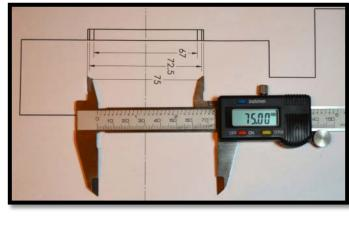
2. Check dimensions to confirm it has been printed to scale.
