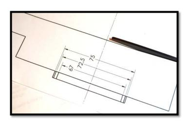
3. Cut the drawing just outside the line. Cut down to hub size of wheel.
