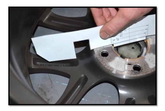
5. Lay the template inside the wheel as shown. Verify that the edge of the caliper does not touch the rim or the wheel spokes. A minimum clearance of 2mm (0.080") is recommended.
