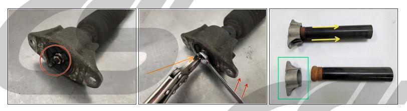
The shock shaft can be easily broken if an impact is used to remove the top nut. We do not recommend using an impact for top hat nut removal.
