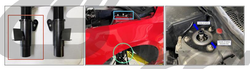
• Locate the front left-hand side coilover. It will appear as shown. The coilovers may be labeled "FL" for front left and/or "FR" for front right.
