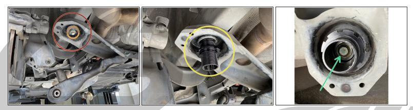
Locate the rear subframe mounting point that is positioned inside the upper spring perch
