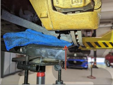
Using a hydraulic jack, lift the knuckle upwards from the lower control arm as shown.
