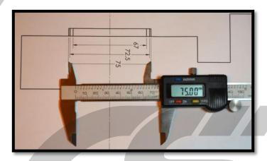
2. Check dimensions to confirm it has been printed to scale.
