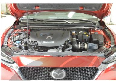
The fully installed FSTB is shown. Re-torque the nuts after a few miles of driving and enjoy!
