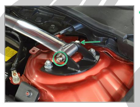
Holding the circled bolt in place with an 8mm allen key, torque the 14mm nut to 23-28 ft. lbs. Repeat step on the passenger side.
