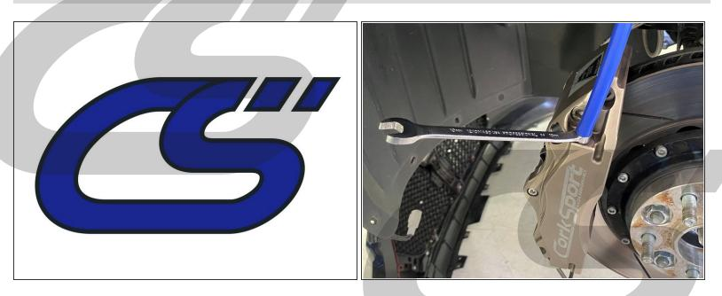
For proper brake bleeding, always start with the bleed screw furthest from the master cylinder. In this case we start with the outer bleed screw on the passenger side, then work your way inward going to the inside Caliper Bleed Screw, then the Parking Brake bleed screw
