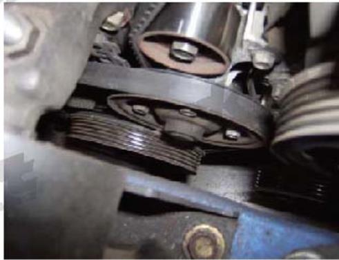
Step 26: Reinstall power steering/A/C belt and tighten.
