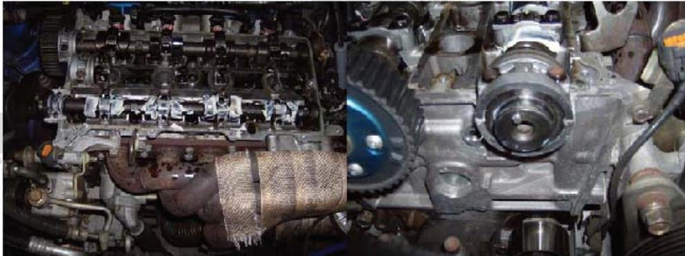
Step 16: Apply small amount of silicone sealant to flange surface of front cam cap and install all cam caps in the order and direction noted when removed and tighten from the center cap outward in 2-3 steps. Tighten to 100-125in/lbs.
