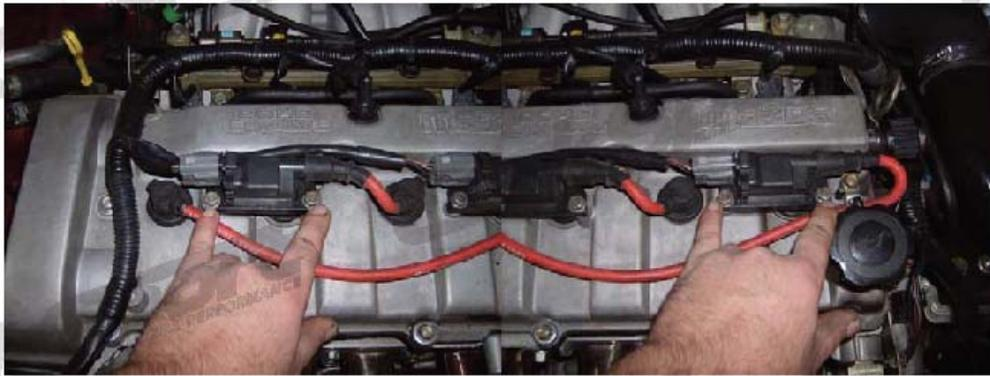
Step 28: Reconnect cam sensor, crank sensor, power steering and A/C plugs.
