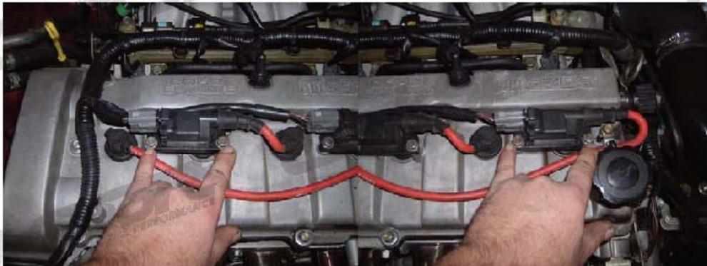
Step 4: Remove the PCV from valve cover. Remove the crank case vent hose from valve cover. Remove the eleven (11) 10mm head bolts from the valve cover and remove valve cover.
