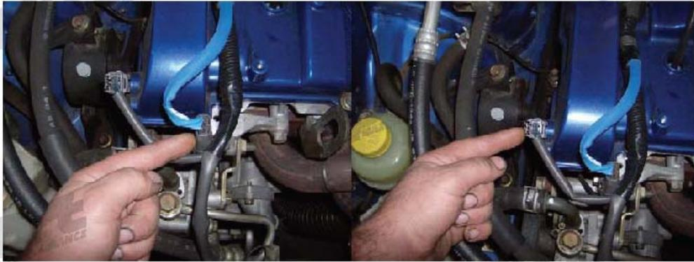
Step 3: Remove two (2) 10mm head bolts from each coil pack and remove coil packs with their high tension leads from valve cover.
