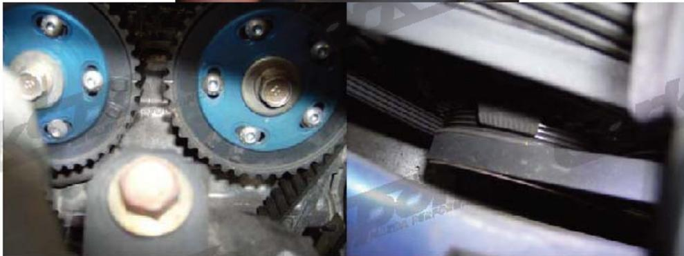
Step 6: Loosen the 14mm head pivot bolt on the power steering pump. Loosen the 14mm head hold down nut on the power steering pump bracket. Loosen the 14mm head tension bolt till the power steering- A/C belt is loose enough to be removed.
