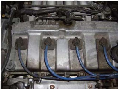
Step 28B: Reinstall power steering lines onto valve cover with their original two (2) 10mm head bolts. Reconnect crank shaft position sensor and re-clip harness to power steering lines.
