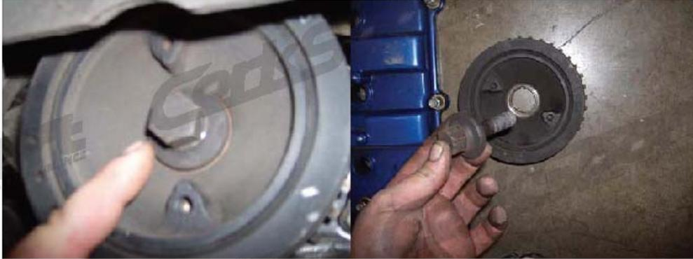
Step 10: Remove the four (4) 10mm head bolts from the plastic lower timing belt cover and remove cover.
