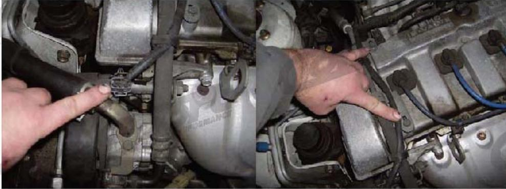
Step 3B: Remove spark plug wires from valve cover by using a slight twisting and pulling motion. Disconnect coil wire from coil and remove two (2) Phillips head screws from distributor cap. Remove cap and set aside.
