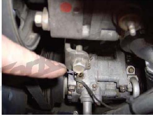
Step 7: Loosen the four (4) 10mm head nuts on the water pump pulley. Loosen the 14mm head pivot bolt on the lower bracket of the alternator. Loosen the 12mm head bolt on the alternator hold down bracket. Loosen the 12mm head belt tensioning bolt till the belt is loose enough to be removed and remove belt. After belt is removed, remove the four (4) 10mm head bolts from the water pump pulley and remove pulley.
