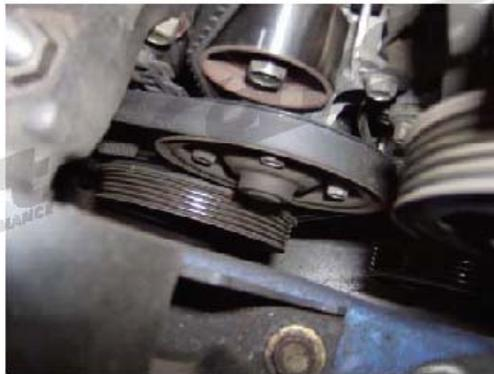
Step 8: Remove the four (4) 10mm head bolts from the plastic upper timing belt cover and remove cover.
