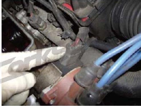
Step 27B: Reinstall plug wires into valve cover.
