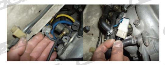
Step 26: Reconnect the colored solenoid plugs to their matching solenoid. Replace the 2 original 12mm head bolts into the tubing rack to block.
