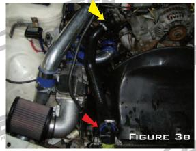
B) REINSTALL THE UPPER SILICONE RADIATOR HOSE AND TIGHTEN WITH THE UPPER T-BOLT CLAMP (38-43MM) SHOWN BY THE YELLOW ARROW IN FIGURE 3B. TIGHTEN THE 47-55MM T-BOLT CLAMP SHOWN BY THE RED ARROW IN FIGURE 3B.
