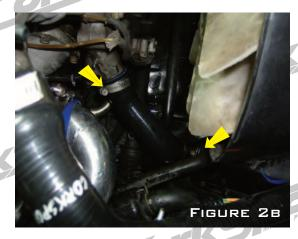
B) REINSTALL THE LOWER SILICONE RADIATOR HOSE AND TIGHTEN WITH THE TWO PROVIDED 38-43MM T-BOLT CLAMPS AS SHOW IN FIGURE 2B.
