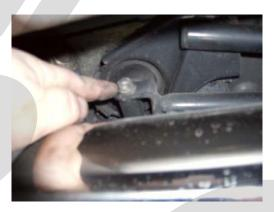
Remove the 12mm headed bolt from the shifter and the linkage and slide the linkage from the shifter. This will free up the entire shift rod to be removed from the car. Slide it backward and out of the car (once it clears the front subframe, it will be free to come out around the side of the exhaust piping.)
