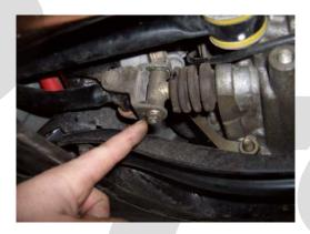
**Step 3:** Remove the shift linkage bolt by pulling it up and out.
