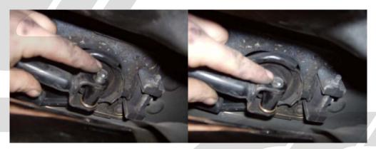
**Step 17:** Reinstall the 12mm headed bolt on to the shifter and tighten to 12-16 ft/lbs of torque.
