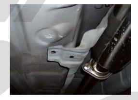
**Step 7:** Remove the 12mm nut shown below from the shifter.
