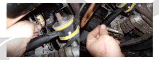
**Step 4:** Slide the shift linkage back from the transmission.
