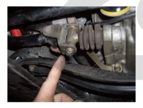
**Step 16:** Slide the shift linkage back in place at the shifter and reinstall the 12mm headed bolt.
