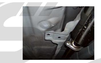
Step 11: Remove the 12mm nut shown below from the shifter.
