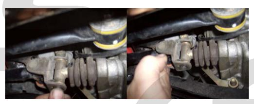
Step 8: Reinstall the 12mm headed nut and tighten to 12-16 ft/lbs or torque.
