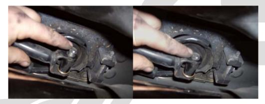
Step 16: Reinstall the 12mm headed bolt on to the shifter and tighten to 12-16 ft/lbs of torque.
