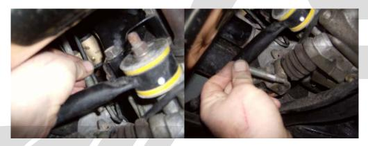
Step 4: Slide the shift linkage back from the transmission.
