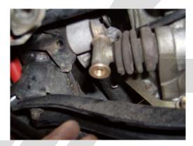
Step 7: Slide the shift linkage over the transmission linkage and replace the bolt from the top.
