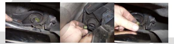
Step 14: Install the two remaining bronze shifter bushings into the shifter.
