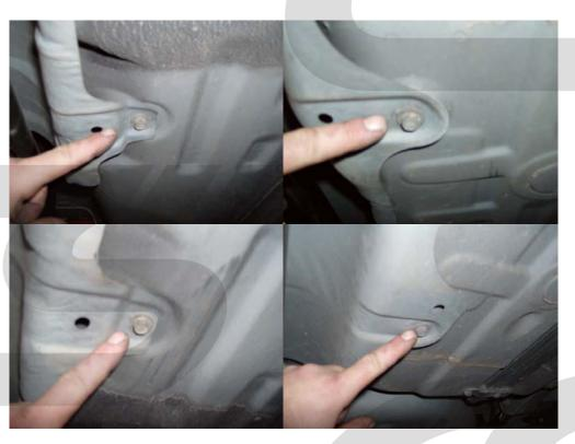
Step 10: Slide the heat shield back several inches to gain access to the shifter.
