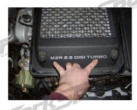
Step 3: Disconnect MAF sensor. Loosen hose clamp at air box with 10mm wrench or Phillips head screw driver. Unclip the air box cover and remove cover.
