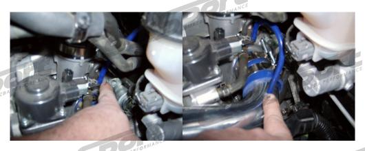
Step 14: Connect supplied 14mm silicone hose onto 14mm nipple on inlet pipe and onto crank case vent tube on valve cover. Depending on Routing you may want to trim some of the silicone.
