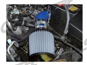
Step 21: Remove two (2) Phillips head screws from MAF sensor on stock air box cover and remove sensor. Install MAF sensor into MAF housing, making sure that the sensor is fully seated prior to installing and tightening the two (2) 3mm Allen head bolts. Reconnect MAF sensor plug.
