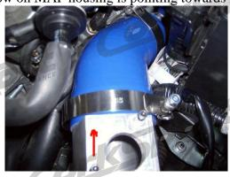
Step 20: Install supplied air filter onto end of MAF housing and tighten its clamp. Position Silicone coupler as shown and tighten remaining T-bolt clamps.
