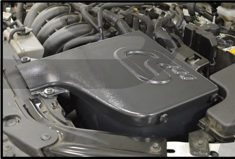
**Thank you for purchasing the CorkSport Cold Air Box.** Protect your short ram intake from excessive engine bay heat with our two piece cold air box. CAD designed and thermoformed this box fits like it was suppose to be there from the factory. Utilizing all the OEM mounting points and shipped with supplied hardware installation of this box is a breeze.
