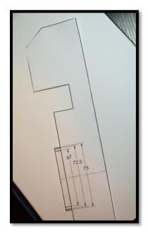
4. Glue the drawing to a stiffer piece of material such as a manila folder to make the template easier to use. Finish by cutting directly along the line.
